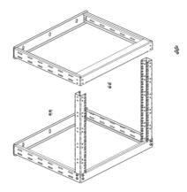
Step 3 Attached the right-side and left-side support straps by securing 4 of the M6x12mm Phillips head screws and M6 nut to the top panel frame and vertical mounting rails.
