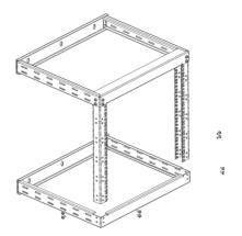
Step 2 Insert the other end of the vertical mounting rails into the corners of the top panel frame opposite the mounting side and secure them with 2 of the M6x12mm Phillips head screws and M6 nut on each side.
